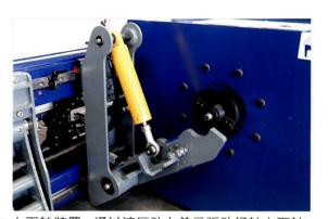
▲ 上下轴装置:通过液压动力单元驱动经轴上下轴,额定负载高达 4000KG Load/unload device: Driven by hydraulic power unit, rated load up to 4000 KG
