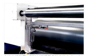
▲ 上油上蜡装置:倒轴时可采用多种穿纱方式,减少了中间过渡罗拉的摩擦。 Oiling/waxing device: various types of yarn threading methods when beaming, reduce friction of middle guide rollers
