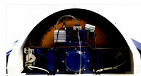
▲ 制动系统:采用液压盘式制动器,制动快速平稳 Brake system: Hydraulic disc type brake, fast and stable
