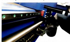
▲ 导轨排布: 二条高精度直线导轨,分布在撑挡内外二侧面 Guide rail: Two high-precision linear guide rails, installed on each side of the wall
