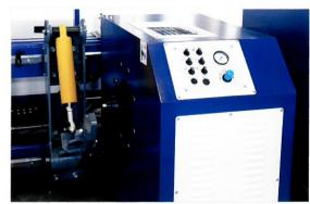
▲ 拍开拍合:齿轮箱左右移动实现拍开拍合 Clap/unclap: Achieved by gearbox moving leftward & rightward
